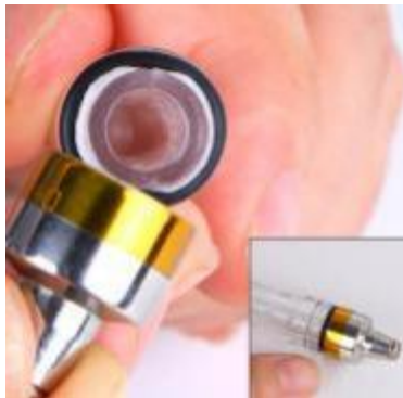
Connect the probe tightly with the PVC vacuum hose
