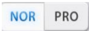
RF Mode Selection (NOR is the set mode. The red LED is on and energy is at the set level and stay at the set level after turning on the device. PRO is the smart mode. The red LED stays on once switch on the machine, and the temperature goes up slowly to the set energy after the probe comes in full contact with the skin. )
