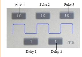
Pulse1: working time of the first pulse, 1-10ms adjustable.
